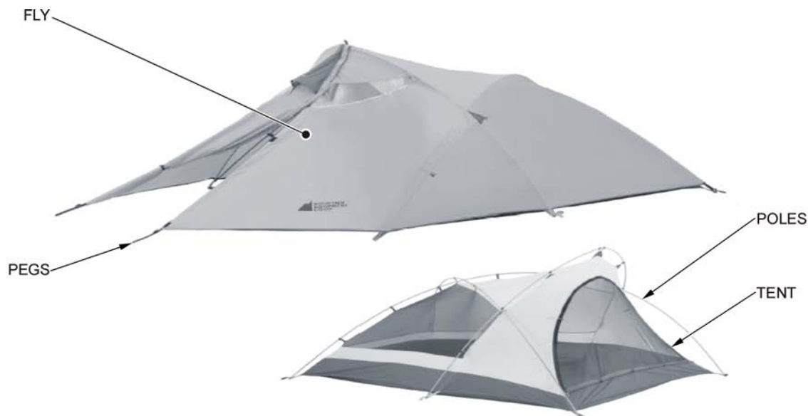
Figure 10-7-1 Sample Tent with Labelled Parts (No Guy Lines)
